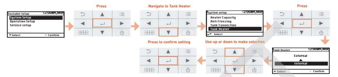
When set to "External, "Tank heater ON time" must be set. This is the delay time that the system will wait, after beginning a DHW cycle, before automatically engaging the booster heater.
