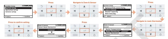
iii. Room Thermostat (Internal): Controlled using the heat pump remote controller as the room temperature sensor.
