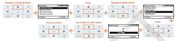
**b)** Tank Heater: This setting enables the backup heater or booster heater (which ever it is set to in system setup) to activate in DHW mode. If set to "No", it will never activate.
