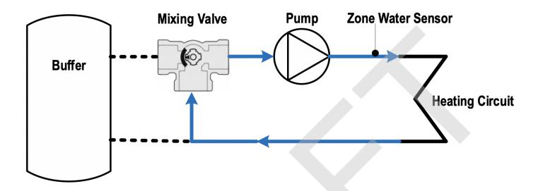
**Mixing:** The valve is open to both the buffer and return from the circuit. The flow temperature is blended down to the required temperature. The valve regulates itself to maintain a steady temperature.
