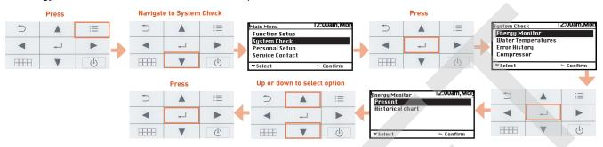
b) Water Temperatures: Shows current outlet/inlet etc temperatures.
