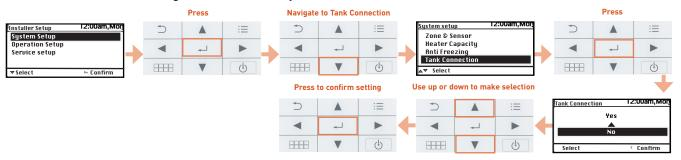
**d)** Tank Heater: This setting tells the system whether to use the built in "backup" electric heater (internal to the heat pump) or DHW tank "booster" (immersion) heater (external to the heat pump) for DHW electrical assistance.
