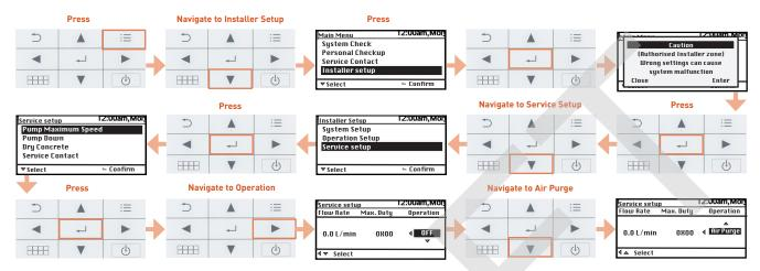
b) Set maximum pump speed: Use the flow rate display. The numbers are shown in hexadecimal and simply refer to the pump duty. Increase or decrease until the desired flow rate is shown, this will be the maximum pump speed.
