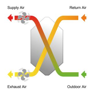
HEAT EXCHANGER DIAGRAM
